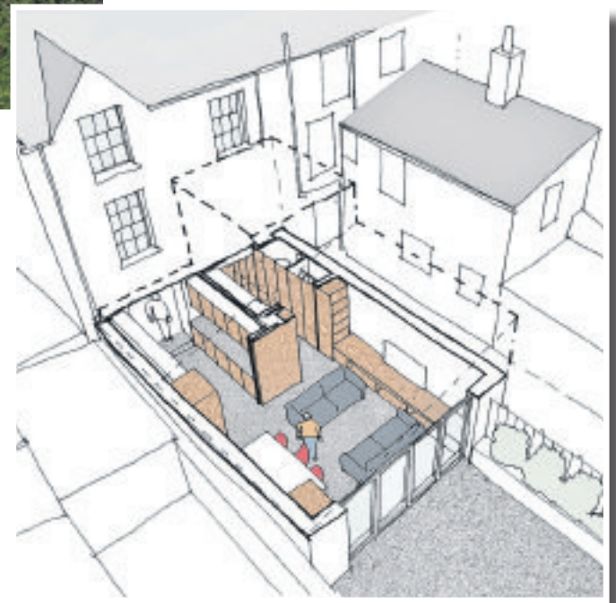
A sketch showing the new living spaces to the rear of the terrace
