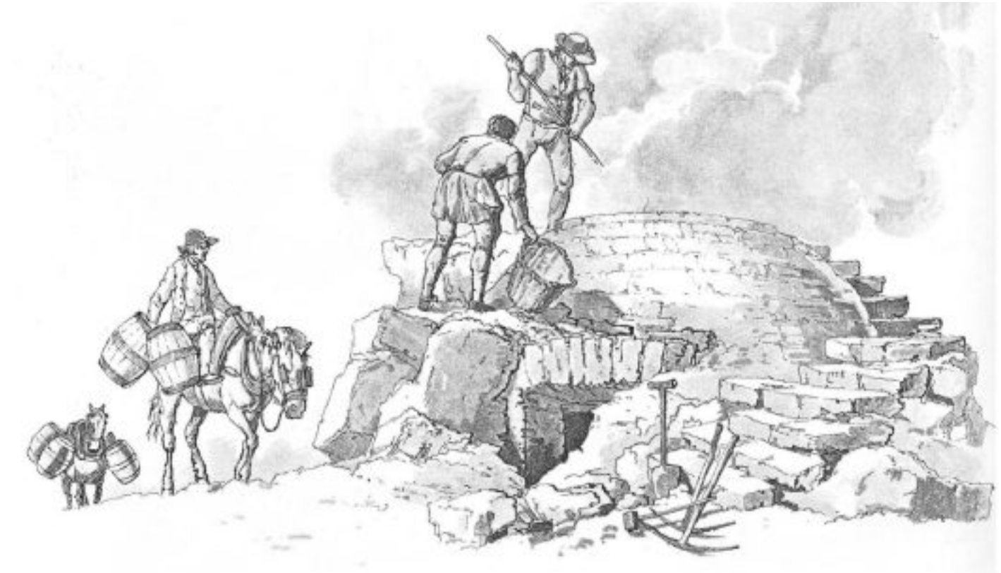
A limekiln, drawn in England about 1805 by WH Pyne. Limestone, broken with the tools in the foreground, and fuel would have been carried up the spiral steps to be loaded in layers into the kiln through the charging hole at the top. The fire would be started from the bottom, and the lime would be raked out from the same opening once the burn was completed. The customer arriving on horseback is bringing his empty barrels to collect quicklime. Note: the free-standing (but vegetation cloaked) limekiln on the Ayres below Ballagarret is of similar construction, but has a ramp to facilitate loading
