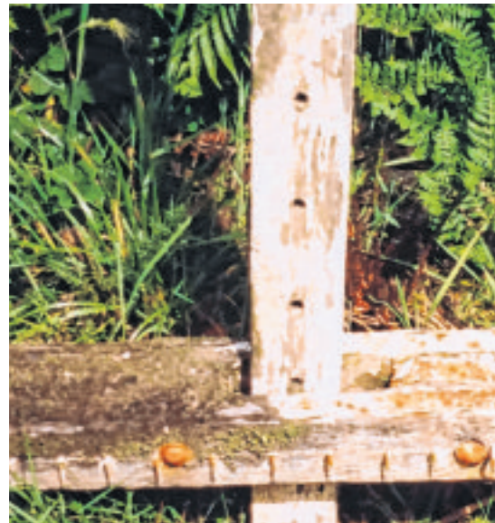
Adjustable bottom rail of a tenter frame at Tynwald Mills
