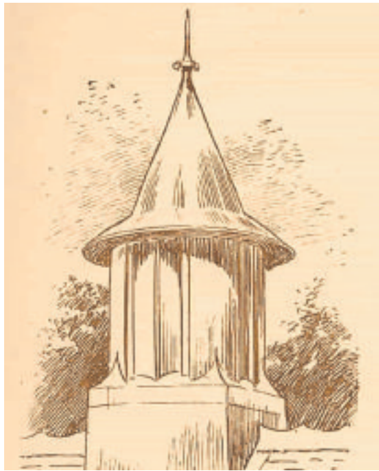
Boyle's patent air-pump venturi ventilator, as originally fitted at the Ward Library
