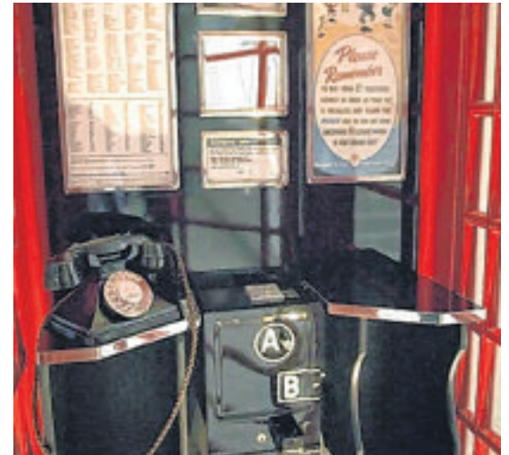
A and B coin mechanism inside a 'Jubilee' K6
