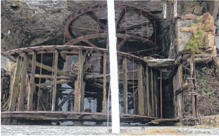
Twin water wheels – larger for the corn mill, small for threshing mill
