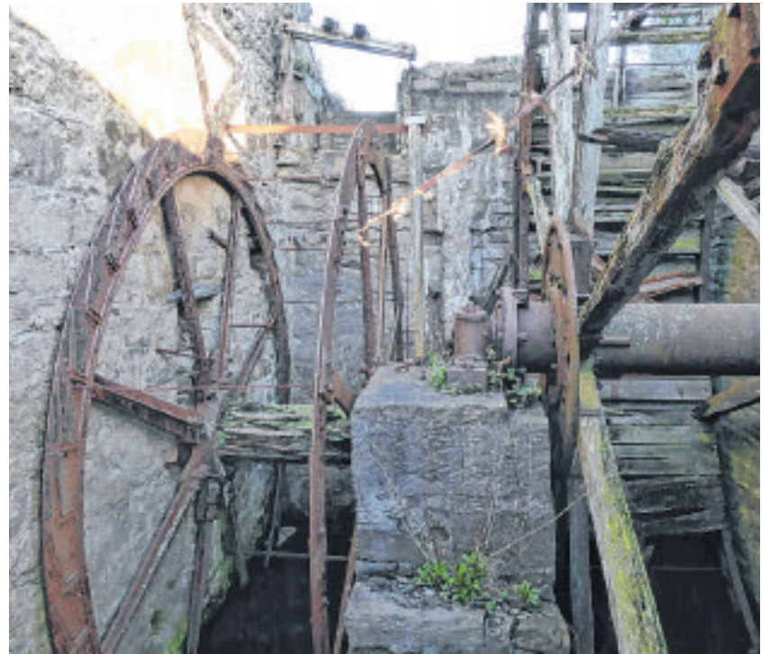
Twin waterwheels at Golden Meadow Mill – smaller one for threshing, larger one for grinding the corn
